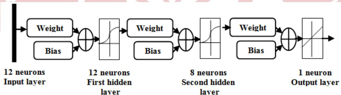
Figure 4: Architecture of ANN Based Fault Detector
