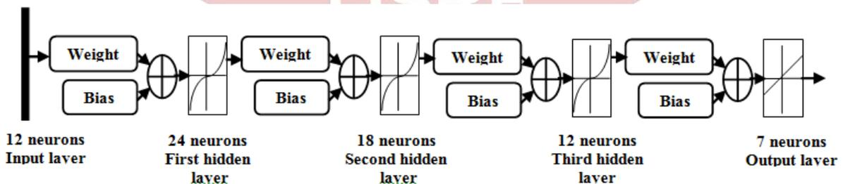
Figure 5: Architecture of ANN Based Fault Classification
