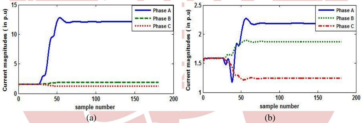
Figure 2: (a) Current signal magnitude of faulty circuit-1 (b) Current signal magnitude of healthy circuit-2 under A1G fault at 10 km with  $R_f = 10\Omega$ ,  $\Phi_i = 90^\circ$
