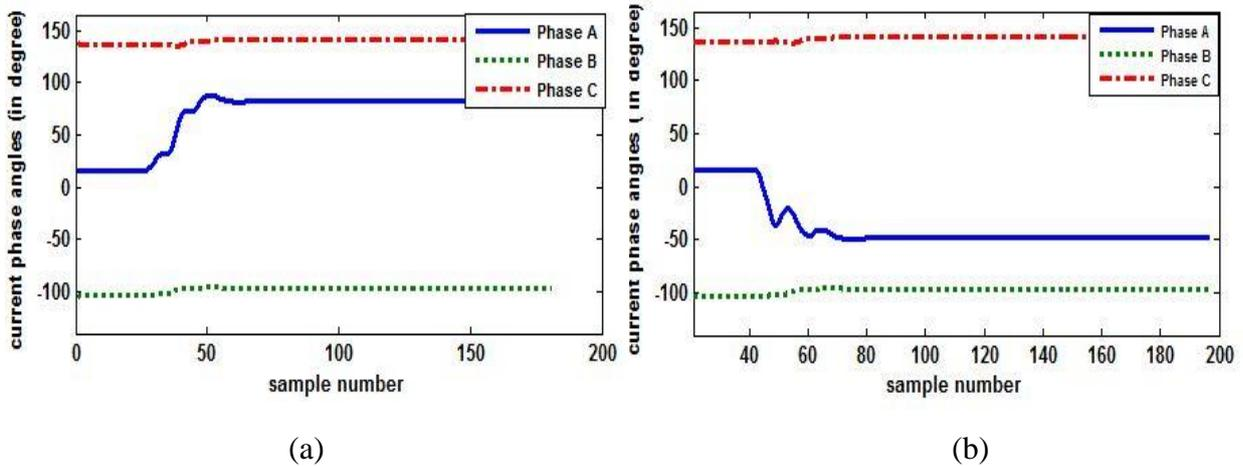
Figure 3: (a) Phase angle of current signals of faulty circuit-1 (b) Phase angle of current signals of healthy circuit-2 under A1G fault at 10 km with  $R_F = 10\Omega$ ,  $\Phi_i = 90^\circ$
