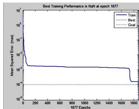
Figure 7: Mean-square error performance of network for fault classification
