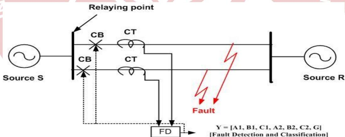
Figure 1: Single line diagram of power system model under study
